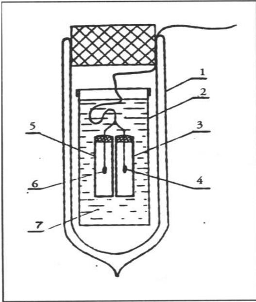
Figure 1. Design of the screened microcalorimeter.
